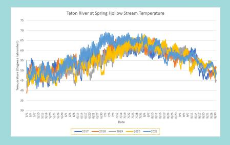
Beginning in 2011, FTR started installing remote temperature loggers throughout the Teton River Watershed. During the fall of 2021, FTR collected temperature data at the 36 temperature loggers currently maintained in the watershed. These loggers are located in all of the major tributaries to the Teton River, along the length of the upper Teton River, and in the Teton River Canyon. By monitoring water temperature, FTR can actively assess impacts on stream conditions and the fishery.
