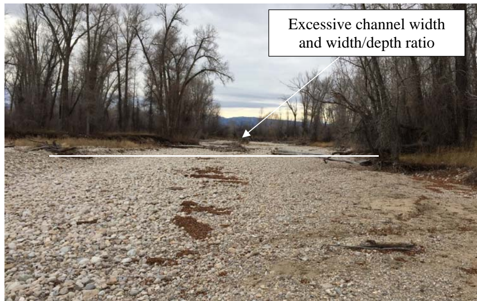
Figure 11. Photograph 9, high width/depth ratio homogeneous channel, Station 47+00 ft.
