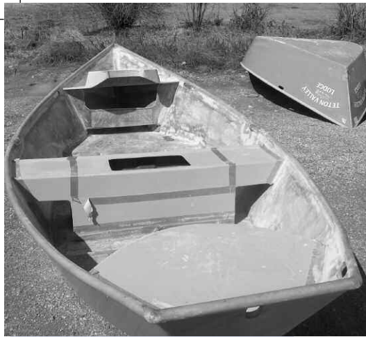
Nearing completion, molds for seating and standing are fiberglassed into place before finishing touches and a paint job.
