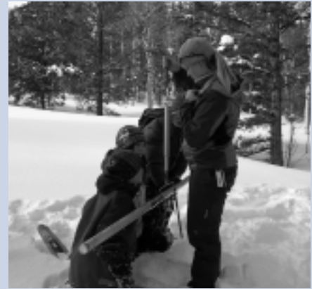
Left: Mike Lien installs a staff flow gauge measurement device on Trail Creek; Right: Anna Lindstedt measuring the snowpack at the Pine Creek Pass Snotel site.
